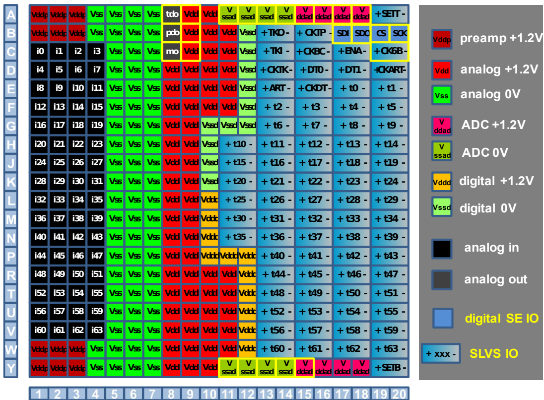
Figure 7: VMM3a pinout (top view)
