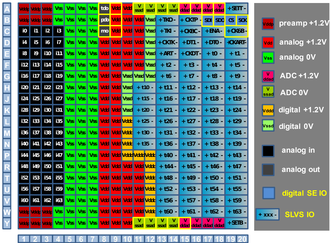
Figure 3: VMM3a pinout (top view)
