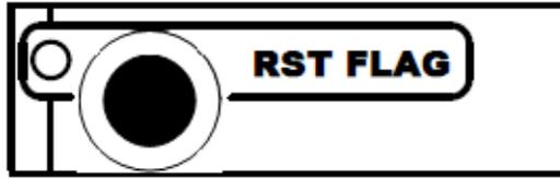
RST FLAG (RESET FLAG) output signal is TRUE (and relevant red LED on) after a RESET occurred, according to the user's settings. The type of reset which asserts RST FLAG TRUE can actually be selected via software.
