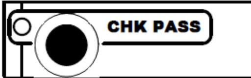
CHK PASS (CHECK PASSED) output signal is True (and the relevant green LED on) when the initial check of the system is successful and the system is ready.
