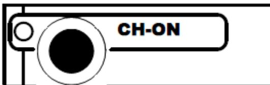
CH-ON (CHANNEL ON) output signal is True (and the relevant red LED on) as at least one board channel is ON (i.e. the channels are enabled and the POWER parameter of that channel is set to ON).
