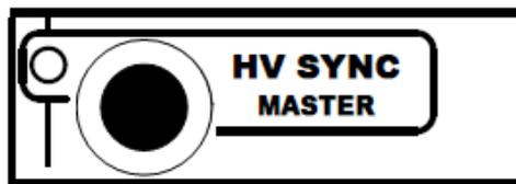
HVSYNC is the synchronisation clock for the Power Supply Units (RS485 standard, 1.25 MHz). It can work either as MASTER (MASTER red LED on), i.e. the synchronisation clock is internally generated and the HVSYNC connector works as output, or as SLAVE (red LED off), i.e. the synchronisation clock is externally generated and sent through the HV SYNC connector which works as input.
