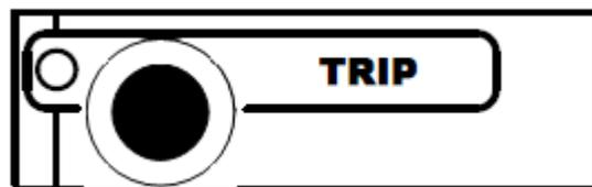
The TRIP output signal is asserted True (and the relevant red LED is lit up) as the status of External Trip line 0 is HIGH (see p. 42); therefore the TRIP condition occurs as at least one channel, latched on External Trip line 0, has tripped and has been switched off due to an Over Current condition. To recover from this state, it is sufficient to turn the tripped channel On again or to execute a clear alarm command via software.
