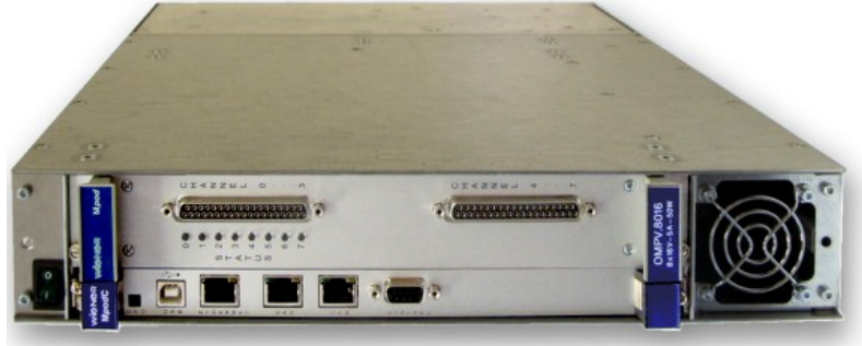
MPOD micro crate with MPOD controller and one low voltage module
